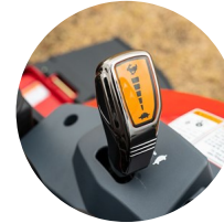
1. 2 range hydrostatic transmission (HST)
