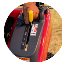
1. PTO lever for mid- and rear rpm
