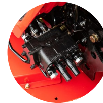
2. 3rd function for 4-in-1 bucket work
