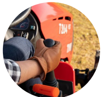
6. Joystick control for front loader
