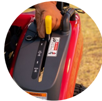
1. PTO lever for mid- and rear rpm
