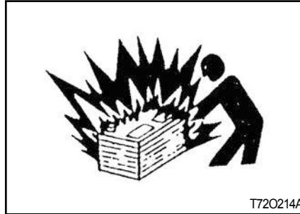
Keep sparks, lighted matches, and open flame away from the top of battery. Battery gas can explode. Never check battery charge by placing a metal object across the poles.
