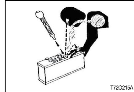
Sulfuric acid in battery electrolyte is poisonous. It is strong enough to burn skin, cause holes in clothing and cause blindness if found entry into eyes.
