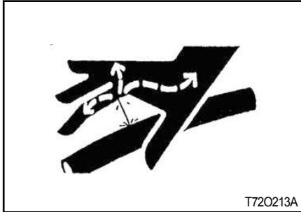
Escaping fluid under pressure can penetrate the skin causing serious injury. Keep hands and body away from pinholes and nozzles, which eject fluids under high pressure. If any fluid is injected into the skin. Consult your doctor immediately.
