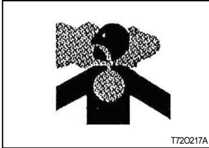
Do not start the tractor in an enclosed building unless the doors & windows are open for proper ventilation, as tractor fumes can cause sickness or death. If it is necessary to run an engine in an enclosed area remove the exhaust fumes by connecting exhaust pipe extension.
