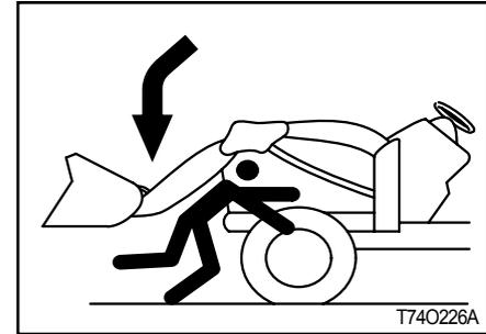
Do not stand under the lifted loader or get close to it. Also, lower the loader arm onto the ground before leaving the tractor. Otherwise, it may lead to a fatal injury or even death.
