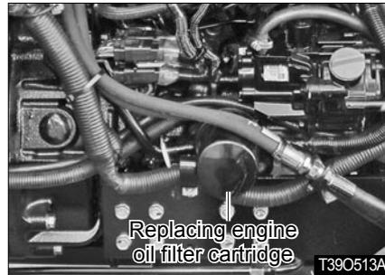
► **REPLACING ENGINE OIL FILTER CARTRIDGE**
