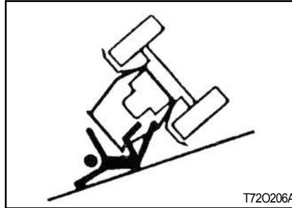
Do not drive where the tractor could slip or tip.
