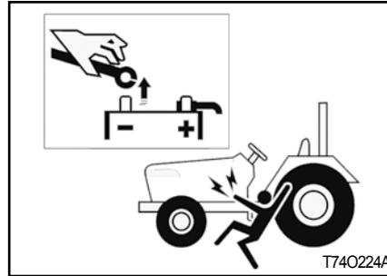
1. When working with your tractors electrical components you must first disconnect the battery cables.
