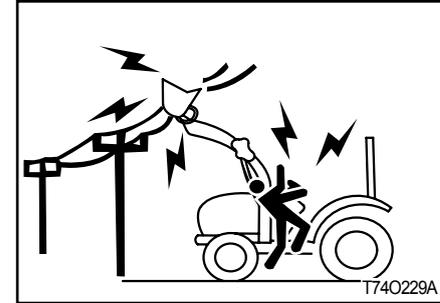
Do not allow loader arms or attachment to contact electrical power lines. Electrocutation will cause serious injury or death.
