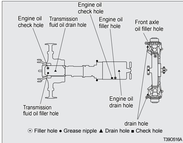
○ Filler hole ● Grease nipple ▲ Drain hole ■ Check hole
