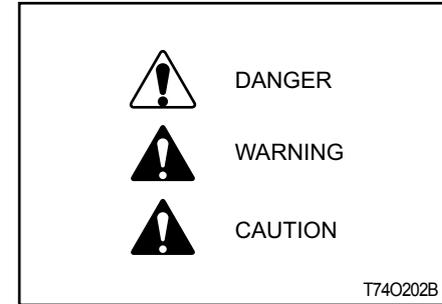
A signal word "DANGER, WARNING OR CAUTION" is used with safety alert symbol. DANGER identifies the most serious hazards. Safety signs with signal Word "DANGER OR WARNING" are typically near specific hazards. General precautions are listed on CAUTION safety signs.
