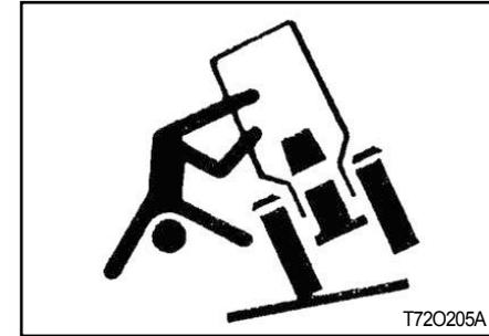
The Roll Over Protective Structure (ROPS) has been certified to industry and/or government standards. Any damage or alternation to the ROPS, mounting hardware, or seat belt voids the certification and will reduce or eliminate protection for the operator in the event of a roll-over. The ROPS, mounting hardware, and seat belt should be checked after the first 100 hours of tractor and every 500 hours there-
