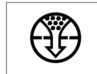
Air cleaner filter contamination warning lamp
