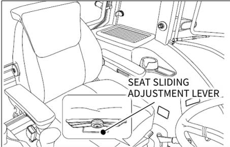
To select seat position, move adjusting lever and slide seat closer to or away from dash panel and controls.
