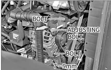
1. Unscrew the Water pump mounting bolts slightly and move the water pump to adjust the tension of the belt.
