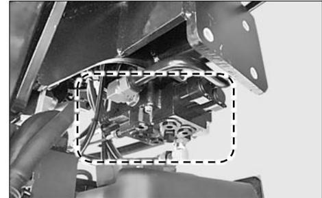
The loader valve is installed under the step on the right side and the joystick lever is installed on the right from the driver's seat in the cabin for easy installation and operation of a loader.
