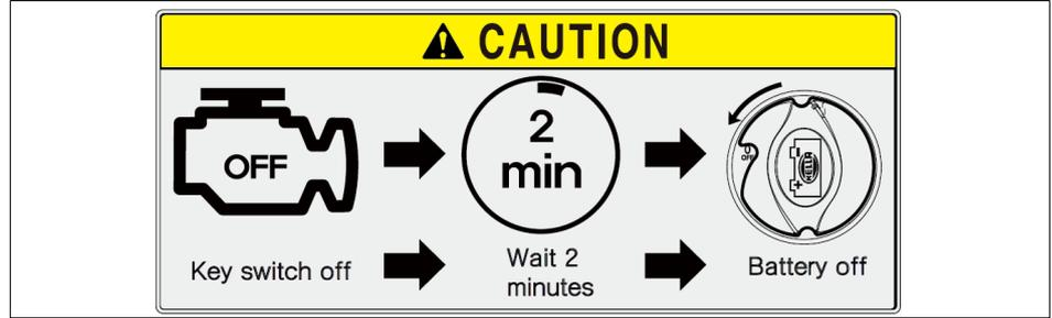
Turn the knob to “OFF” to disconnect the battery and back to “ON” to resume normal operation.
