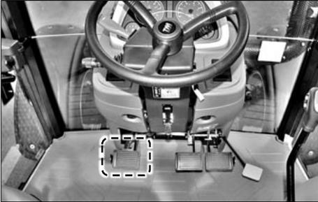
Depressing the clutch pedal disengages the clutch.
