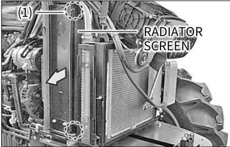
When working in a grassy field or working at night, the radiator or condenser grille may be clogged by grass, straws or bugs, reducing cooling performance. Clean the grill in this case. If dust is stuck between the fin and tube, flush the area with clean water.
