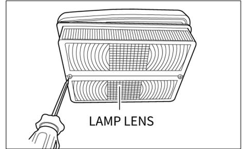
1. Remove the lamp lens using a flat-bladed screwdriver.
