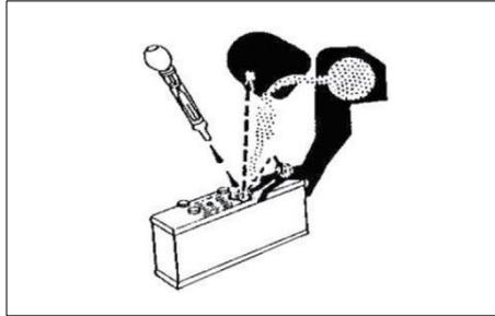
Sulfuric acid in battery electrolyte is poisonous. It is strong enough to burn skin, cause holes in clothing and cause blindness if found entry into eyes.
