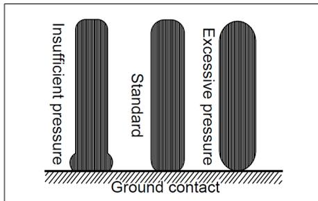
Check if the inflation pressure of the front and rear tires is correct.
