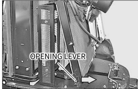
Turn the opening lever to access to the condenser and oil cooler. Clean them with clean water. Remove the grill by unscrewing the pin (1) and moving it in the arrow direction.
