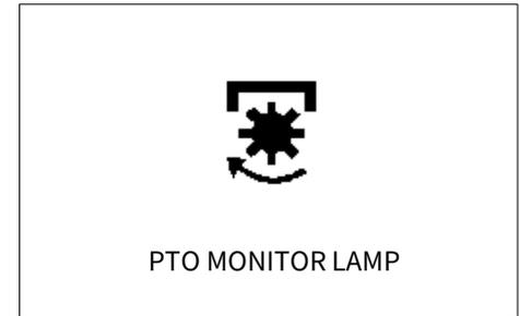
PTO monitor lamp indicates the state of the PTO shaft.
