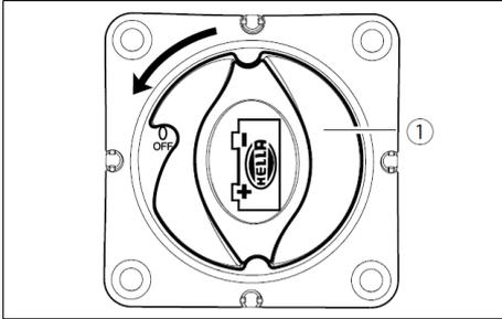
The function of the battery disconnect switch is to disconnect the power supply to the electrical system by interrupting the connection to the battery.
