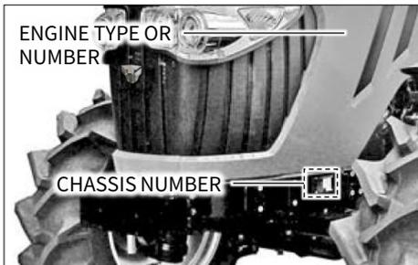
The chassis number is stamped as shown in the drawing above.
