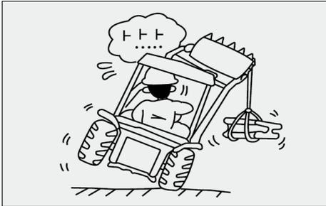
Do not lift anything only with one side of the tractor. If so, the tractor may fall on its side.
