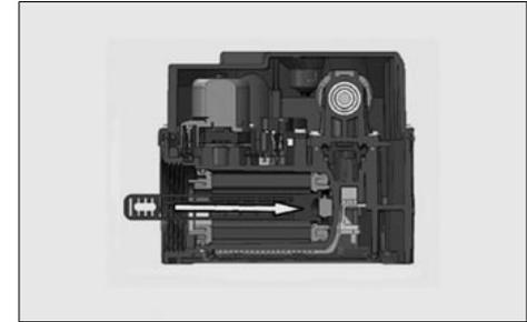
3. Insert the tool till it clips on guide.
