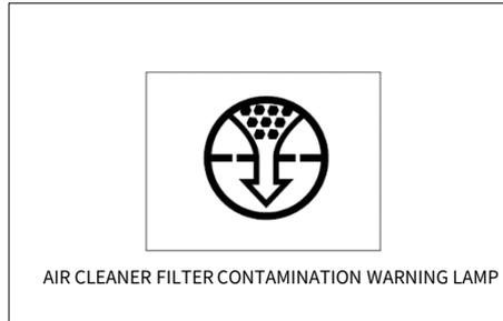
**(30) Air cleaner filter contamination warning lamp**
