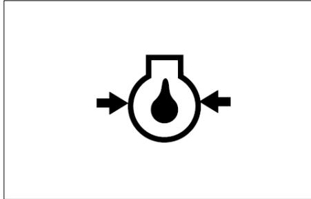
If the oil pressure lamp comes on check the oil level first of all.
