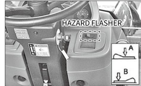
Press the hazard flasher switch in emergency to warn other vehicles in order to prevent an accident. The hazard flasher is operated regardless of the position of the main switch. Also, the turn signal lamp function is disabled while the hazard flasher is activated.
