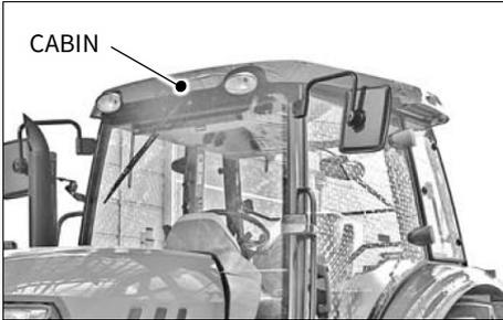
TYM tractors are equipped with a frame for the protection of operators. In the case of cab tractors the frame is incorporated in the cab structure. The objective of the frame or cab structure is to protect the operator in the event of a roll over and they are designed to support the entire weight of the tractor in that event.
