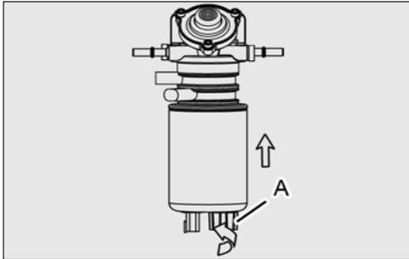
(3) Tighten the drain valve
