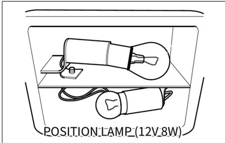
2. Remove the bulb by pressing it and turning it counterclockwise. Fit a new bulb by pressing it turning it clockwise.
