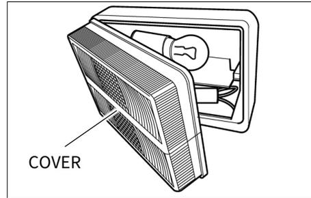
3. Install the lamp lens by pressing it against the cover from one side.
