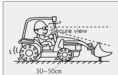
When transporting things with a loader, lower the loader and keep the driving speed slow.
