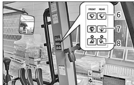
The switches for the windshield/rear wipers/washers and work lamps are located on the right side from the driver's seat.
