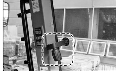
Hold the handle and push it outward to open the window.
