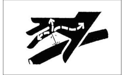
Escaping fluid under high pressure can penetrate the skin causing serious injury. Keep hands and body away from pin holes and nozzle which eject fluids under high pressure.
