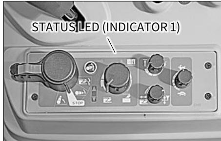
When there is an electric or electronic fault, the indicator (1) blinks according to the setting in the system to inform the type of the fault.
