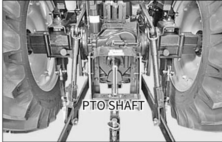
When the PTO shaft is not in use, apply grease and place its cap to it.
