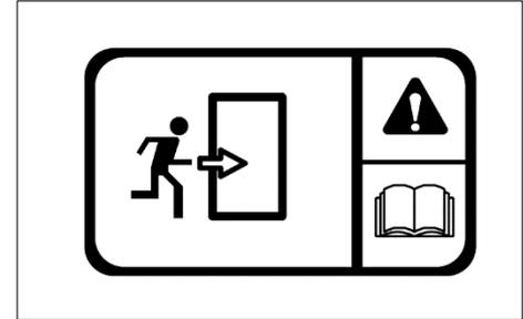
If exit from the cab side doors is blocked (following an accident or vehicle overturn) the alternative safety exits are indicated by decals.
