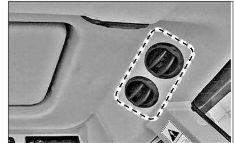
When using the A/C or heater in the fresh air mode, fresh air is drawn into the cabin through the filters installed on the left and right sides of the roof.
