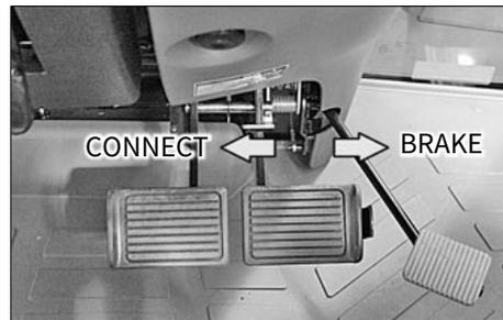
When two brake pedals are installed.
