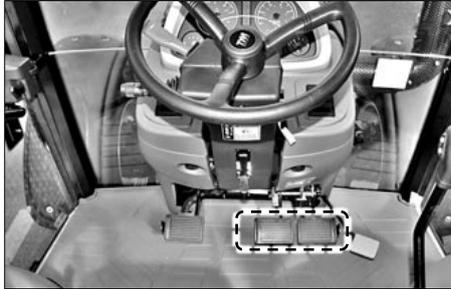
The brake is to stop the machine forcibly.
