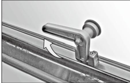
To open the window, push the lever on the center of the rear window in the cabin gently.
