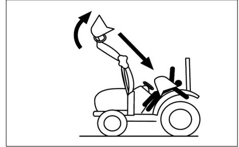
When attaching or detaching the loader, fix all parts which are connected to the bucket and boom. The bucket or boom can be accidentally dropped down, leading to an injury or even death.
