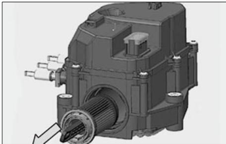
6. Distance of the tool edge from SM when filter is completely demounted : ca. 140.7mm.(5.5inch)
