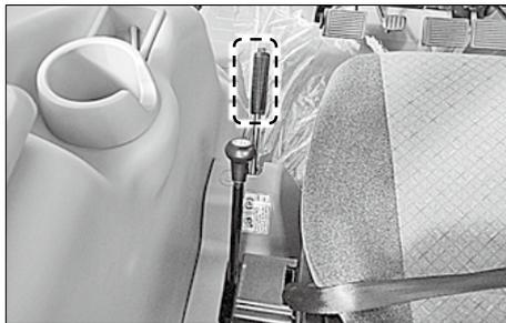
Pull the parking brake lever upward to apply the parking brake. To release the parking brake, press the button at the tip of the lever.
