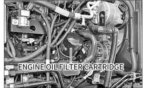
1. Remove the engine oil filter cartridge by turning it counterclockwise with a wrench.
