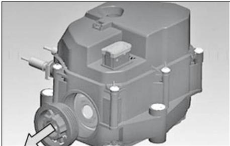
1. Remove the filter cover required.
