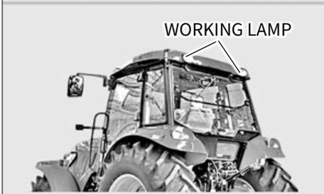
There are 4 work lamps installed on the front and back of the cabin roof. They can be operated by the buttons on the panel on the right side in the cabin.
