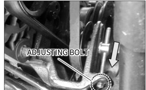
1. Unscrew the alternator mounting bolts slightly and move the alternator to adjust the tension of the belt.
