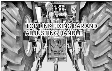
1. The angle of an implement can be adjusted by extending or retracting the top link.
