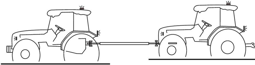
The tractor can be towed only for short distances, such as, for example, from inside to outside a building.
