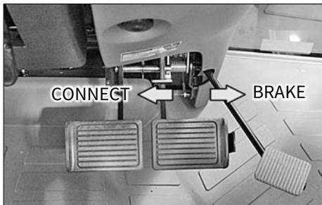
1. Confirm that left and right brake pedals are interlocked when two brake pedals are installed. Make sure to interlock left and right brake pedals unless working in a field.
