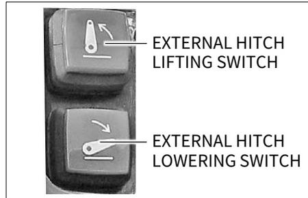
Step 7: When the LED on the Bosch control panel stops blinking, release the external hitch lifting button.
