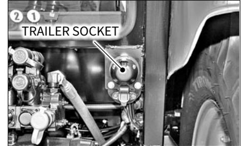
The socket is ready to operate the electrical systems of implements, trailer lighting, warning lamps and etc.
