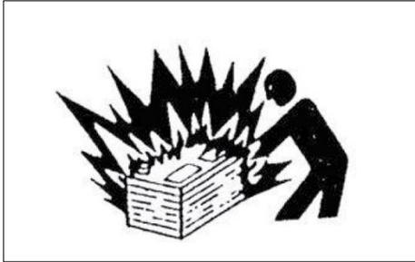
Keep sparks, lighted matches and open flame away from the top of battery. Battery gas can explode.
