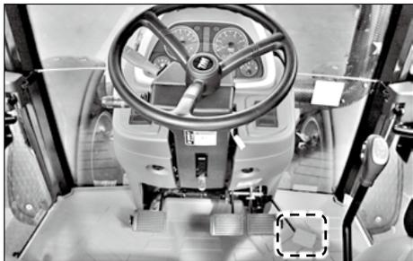
It has the same function to the throttle lever to control the engine speed.
