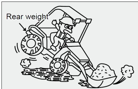
Keep the balance between the front and rear by installing a weight to the back of the tractor or attaching a weight or implement using the 3-point link.
