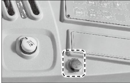
It is possible to use 12v 120w accessory by connecting it to the power socket.
