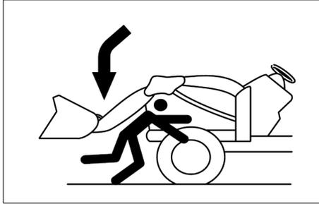
Do not stand under the lifted loader or get close to it. Also, lower the loader arm onto the ground before leaving the tractor. Otherwise, it may lead to a fatal injury or even death.
