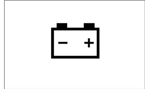
If the alternator warning lamp comes on check all connections and ensure that the fan belt is not broken.
