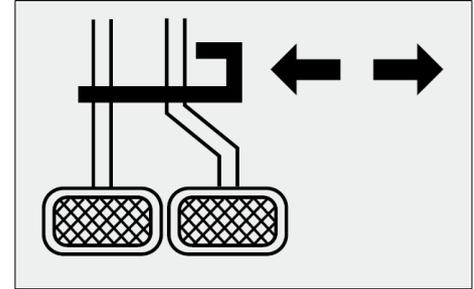
There is an engaging hook for connecting the left and right brake pedals.
