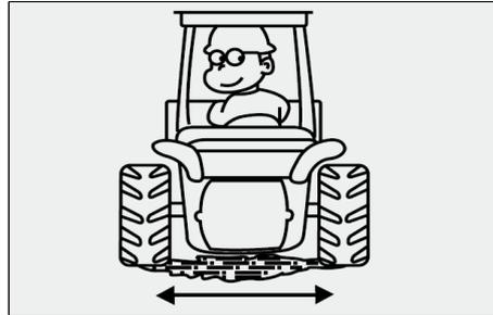
Keep the clearance between the rear wheels as large as possible for safety of the tractor.
