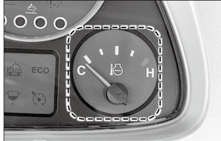
If the needle of the coolant gauge points at "H," stop the engine and check the followings:
