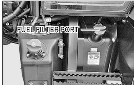
Use only low sulfur or ultra low sulfur diesel fuel.
