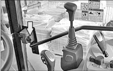
Press the button on the lever to open the door from outside.
