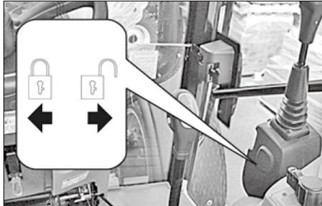
There is a switch to lock the operation of the joystick lever. Pushing it to the left locks the lever while pushing it to the right unlocks the lever.
