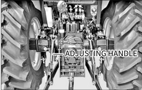
The adjusting link can be adjusted to relieve vibration and shock.
