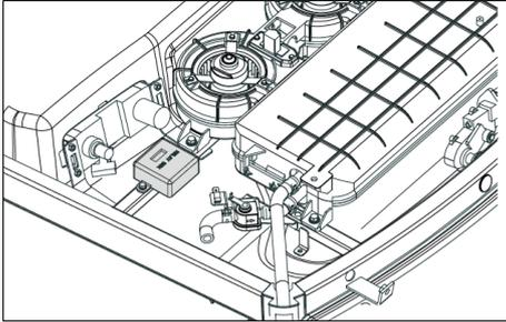
This supplies power to the cabin control panel and cabin electric devices. If any cabin electric device is not operating properly, check this part. If defect is found, replace it with a new one. (The cabin relay box is installed in the roof.)
