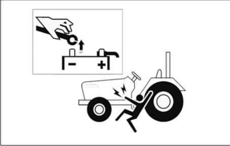
When working with your tractor electrical components, you must first disconnect the battery cables.
