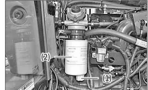
1. Open the drain plug (1) to drain fuel in the filter.
