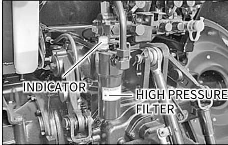
1. When the indicator is turned on in red after the engine is started, the element needs to be replaced.
