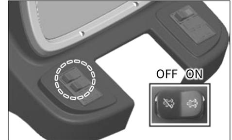
1. **When the Forced DeSOx switch is set in the neutral position, the DeSOx operation is automatically performed for every 200 hours.**
