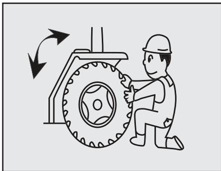
Adjust the wheel tread depending on the type and condition of the work. Also, increase the wheel tread when working on a slope or towing.
