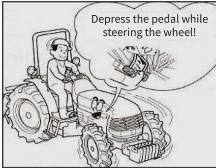
When making a turn, reduce the engine rpm and make a slow turn. When making a turn on the pavement, remove the connector of the brake pedals. Depress the brake pedal on the side to which to make a turn, while steering the wheel, this will allow the tractor to make the turn without moving ahead. Make sure to keep the implement in the up position when making a turn.
