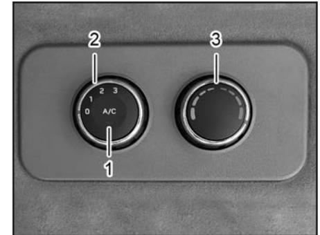
(1) Cooling Function (2) Air Flow Rate
