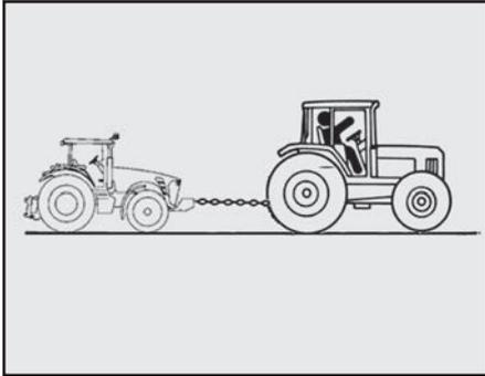
1. Tractor traction should be conducted in short distance. (For instance, from inside to outside)
