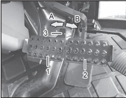
(1) Left Brake Pedal (2) Right Brake Pedal
