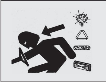
1. When the tractor has an implement attached or is moving slowly, you must often watch the rear side traffic status to avoid a collision accident when travelling on the road. In particular, be careful when you change directions. If necessary, the signal must be given by hand or direction indication lamp must be used.
