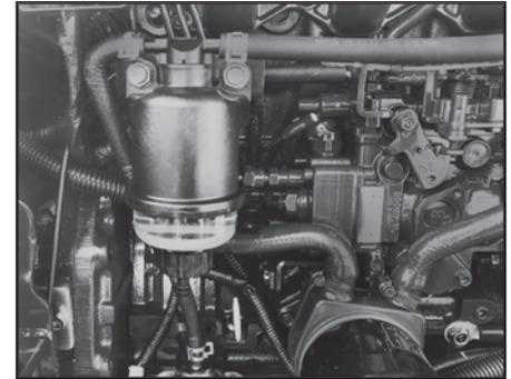
Drain the air from the fuel tank, fuel filter, and fuel filter element when the engine stops as the fuel runs out or during maintenance
