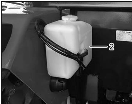
(1) Wiper Switch (2) Wash Liquid Tank
