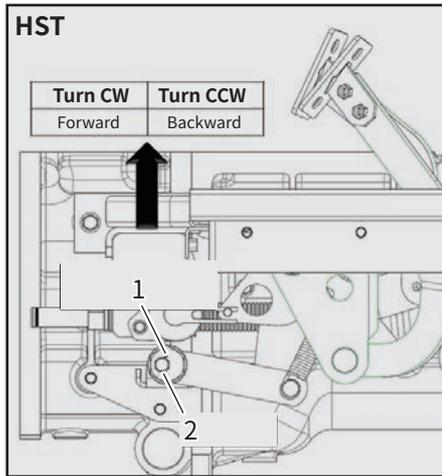
(1) Neutral Adjust Shaft (B) Fix Bolt
