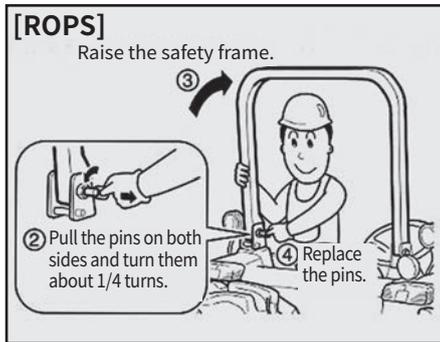
1. Turn the handle to separate the push plate and the ROPS.
