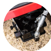
1. Linkage for optional loader
