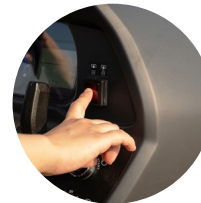
2. PTO on/off switch
