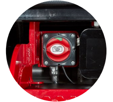
4. Battery shut-off switch
