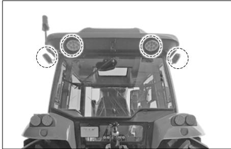
There are 8 working lamps installed on the front and back of the cabin roof, 2 working lamps on top of turn signal lamps and 2 working lamps bottom of head light.
