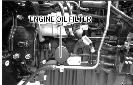
1. Remove the engine oil filter cartridge by turning it counter-clockwise with a wrench.
