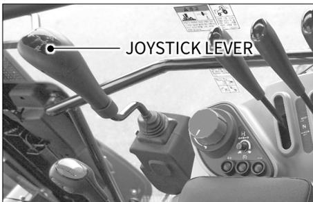
This lever is used to control a loader (when equipped).
