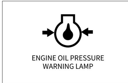
This is illuminated when the engine oil pressure or oil amount is insufficient during driving.
