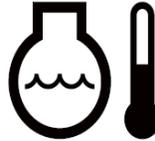
If the coolant warning lamp comes on, the engine is over-heated.
