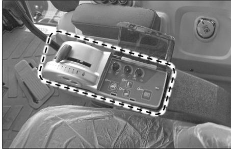
The electronically controlled lift system can provide various functions through simple switch operations, unlike the mechanical type, to enhance the driver's convenience and efficiency.
