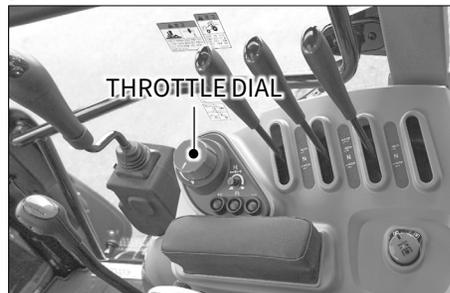
Like the throttle pedal, it is used to control the engine speed.
