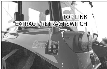
Top link position can be adjusted outside with an external switch installed on the left side of the sub fender.
