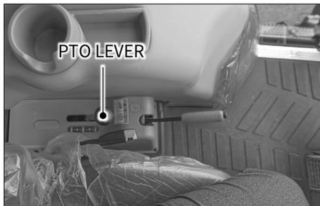
This lever is used to select the PTO speed among 540, 750 and 1,000 RPM.
