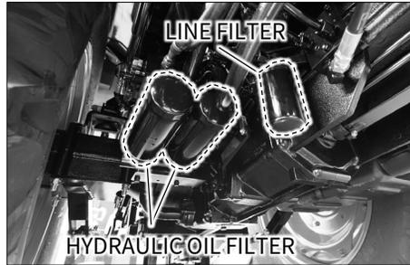
1. Remove the hydraulic oil filter element by turning it counter-clockwise with a wrench.
