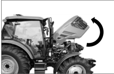
Lift the hood with hands slightly while pushing the lever inside.
