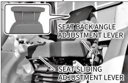
Before operating a tractor it is important to adjust the seat to the most comfortable position & check whether it is properly locked in its position.
