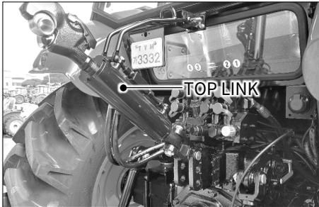
A hydraulic top link is installed on the tractor.
