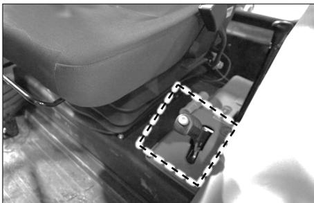
Pull the parking brake lever upward to apply the parking brake.
