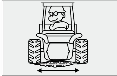
Keep the clearance between the rear wheels as large as possible for safety of the tractor.
