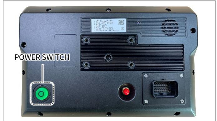
Power switch is used to turn the screen on/off or reboot the system.
