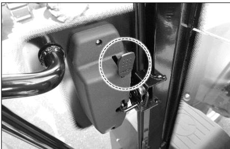
Press the button and pull the lever to open the door from outside.
