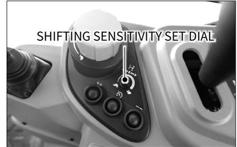
Moving speed of forward or reverse direction at starting can be adjusted using this dial.
