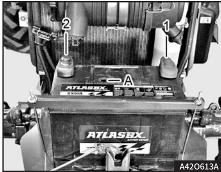
(1) Thick red wire (+) (2) Ground cable (-) (A) Sight glass
