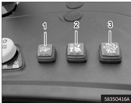
(1) Turn UP Switch (2) Back UP Switch (3) DPF Regeneration Switch
