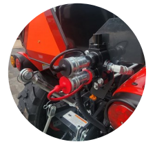
6. 2 port rear hydraulic control (Optional)
