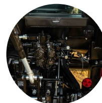
3. 2 sets of rear remote valve for various implements
