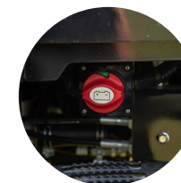
4. Battery shut-off switch
